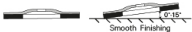
T-27/Flat – For working on flat grinding surfaces. Most efficient when used between 0°-15° angle. The best choice for smooth finishing.
